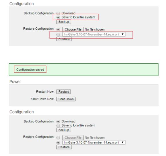
You can also choose "Save to local file system" to save the configuration file in the local drive. Click button to back up. This process normally takes less than a minute as the InnGate gathers the system configuration into a binary file.
